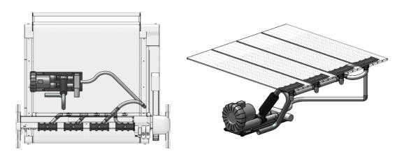
Each table plate has its own **built-in pneumatic vacuum selector**. The selector is driven by the pneumatic valve on the pneumatic front board of the unit.
